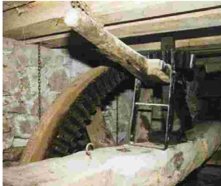
STONENUT DRIVEN DIRECTLY FROM THE PITWHEEL
